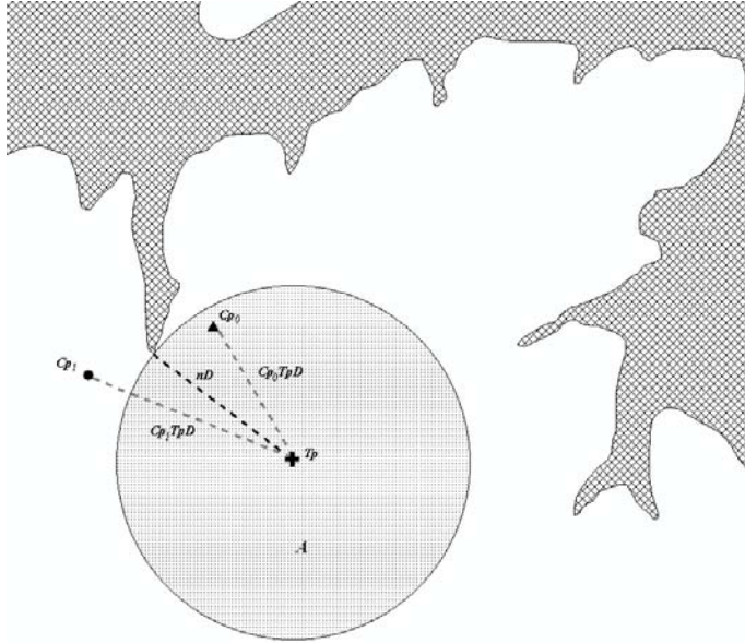
Figure 1: Schematic of the nearest distance to edge heuristic proposition. No point within region A can have a different topological relationship to the polygon than the relationship that Tp has with the polygon.
